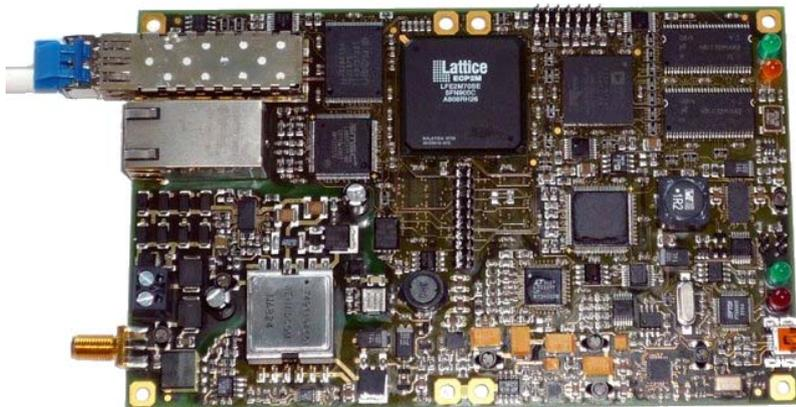
The **RF head** – separate, to allow replacement on site by the customer in a short time. The customer saves time and money when it comes to upgrading, as just the existing 5GHz head and the 5GHz antenna need to be replaced by a new 7GHz head and the appropriate antenna. It is a matter of course that mPOINT is designed as a full duplex transmission system for all bands.
